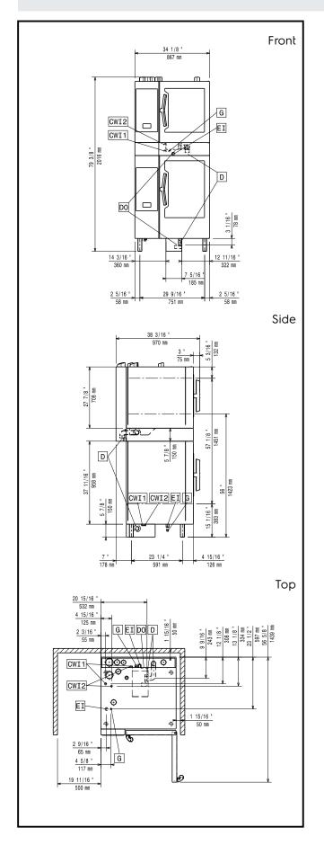
$Installation \ accessories \\ Stacking \ kit for 6 \ GN \ 1/1 \ oven \ placed \ on \ gas \ 10 \ GN \ 1/1 \\$
